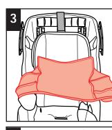
Pull pad off the top of seat and off of headrest.
